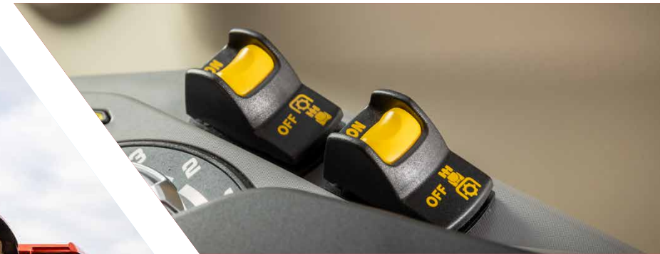
Electro-hydraulic PTO speed selection
