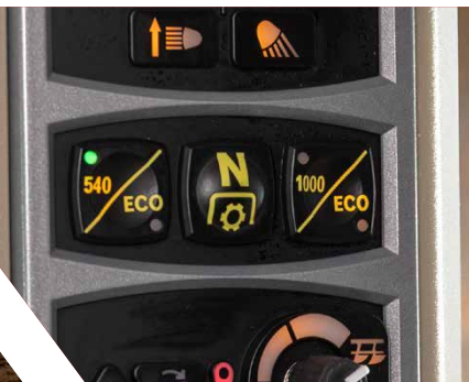
Electro-hydraulic PTO speed selection
