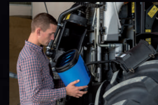
The well proportioned cooling package is easy to access, clean and maintain. 90% of dust is removed naturally thanks to the suction from the cooling fan. The engine air filter is also very easy to access and clean.
