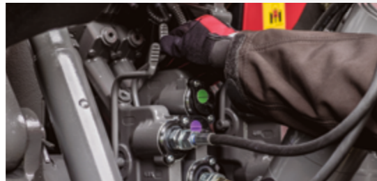
Conveniently located decompression levers
