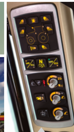
Pillar mounted PTO speed selection controls and linkage controls.
